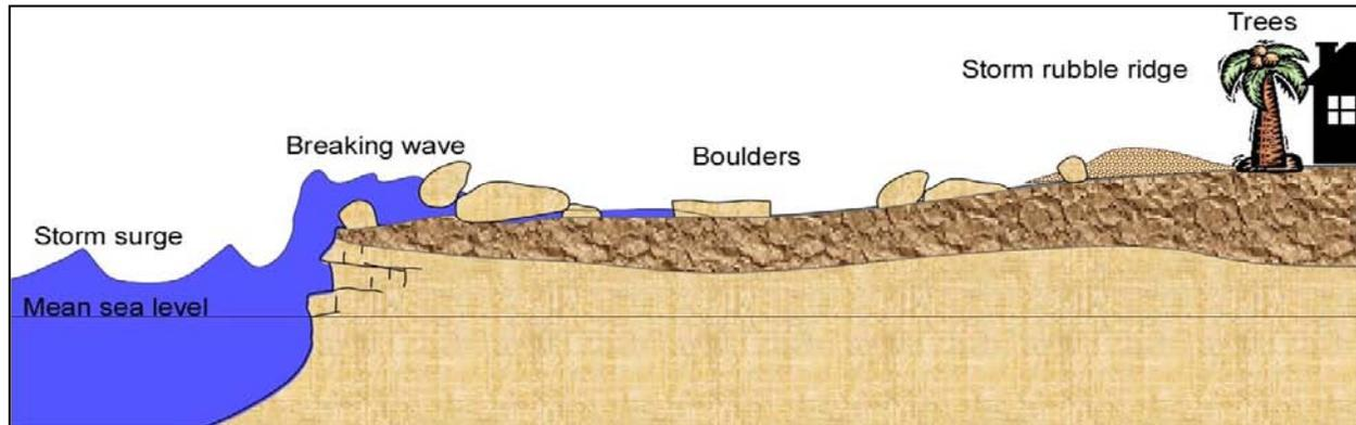
*The calculation of setbacks for permanent structures on coastlines needs to be site-specific. The assessment of waves and associated boulders and debris encroachment inland can be used to assist in assigning site specific setbacks for shoreline construction. Diagram courtesy: Rowe, D-A., Khan, S.A. & Robinson, E., The University of the West Indies Marine Geology Unit.*
