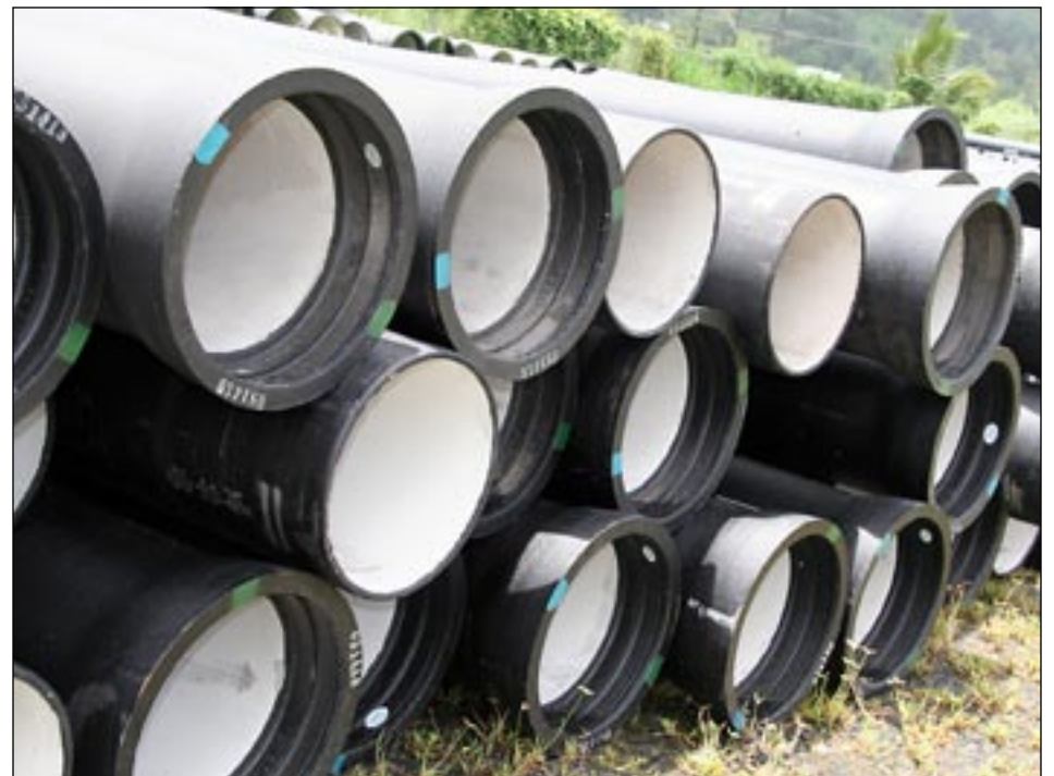
New 20" pipes for water distribution
